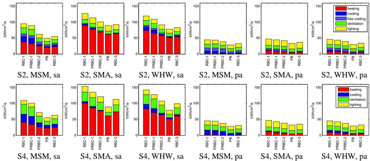
Figure 5. Average annual total NRPE usage for heating (by radiators, floor heating, mechanical ventilation), cooling (by chilled ceiling, mechanical ventilation), free cooling, ventilation (by fans) and lighting depending on control strategy.
