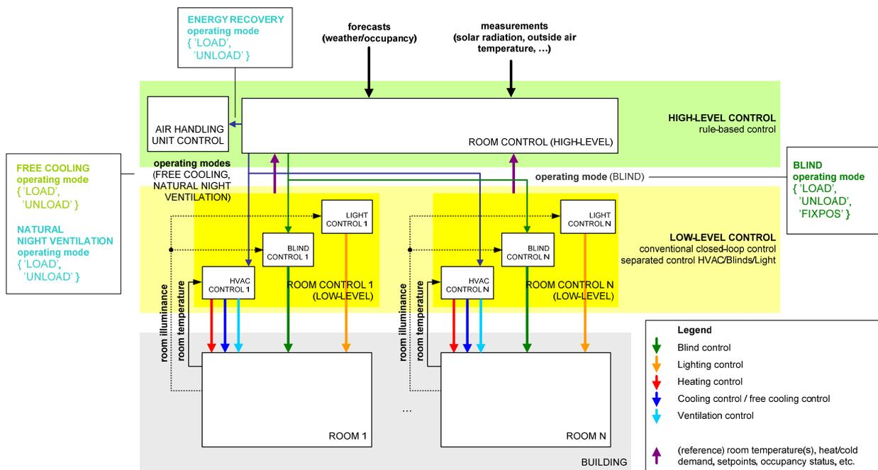
Figure 2. Schematic representation of present-day IRA control solutions [13]. Note, only a subset of the signals involved is displayed.
