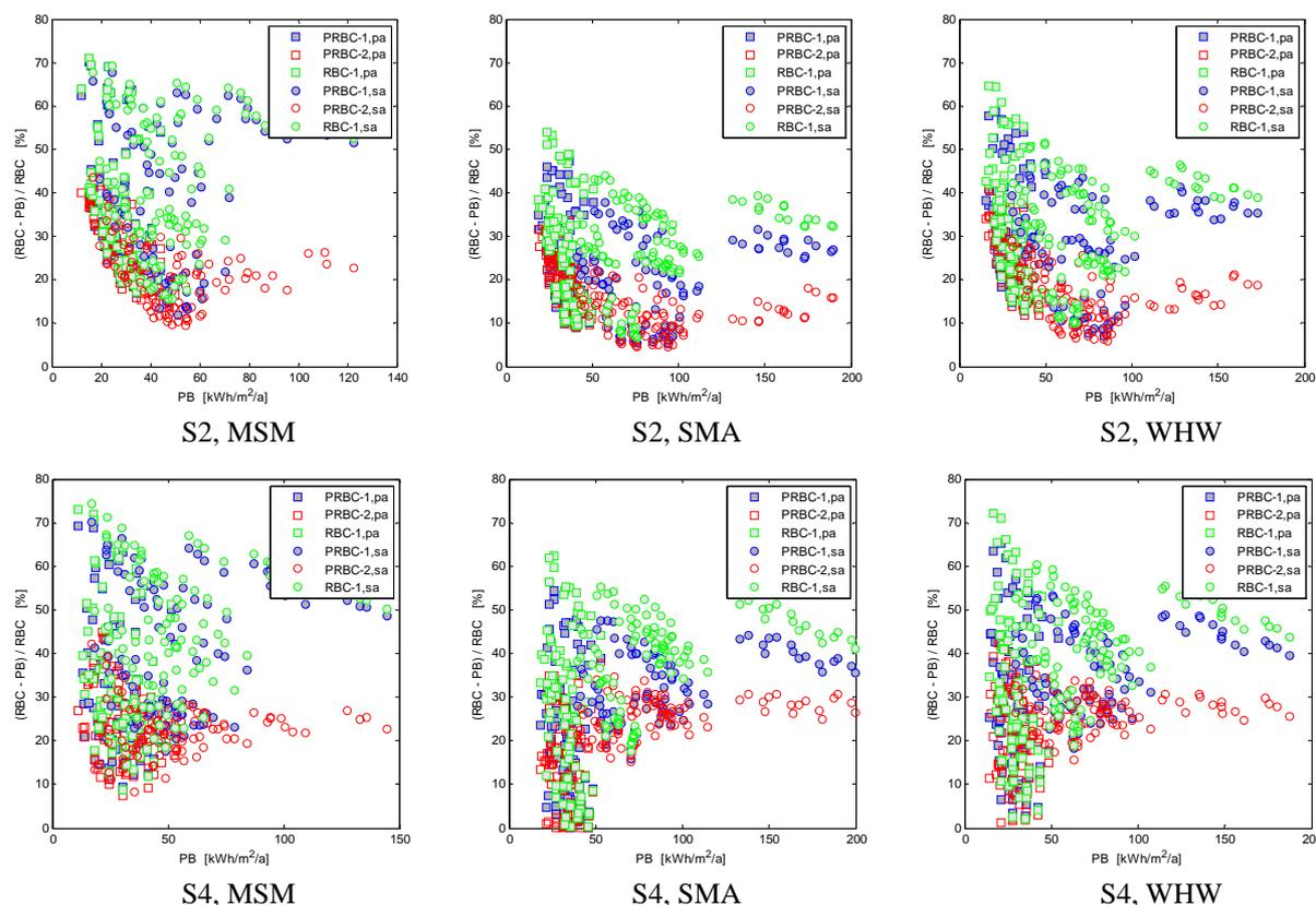
Figure 3. Relative additional annual total NRPE usage for control algorithms RBC-1, PRBC-1 and PRBC-2 compared to the PB.
