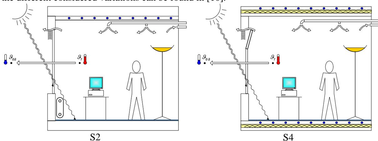
Figure 1. Building systems S2 and S4 [10]. S2: blinds, electrical lighting, radiators, chilled ceiling (with cold from chiller or from free cooling), mechanical ventilation. S4: blinds, electrical lighting, floor heating, (controlled) natural night-time ventilation, mechanical ventilation.  $G_{0a}$ : outside air temperature,  $G_r$ : room temperature
