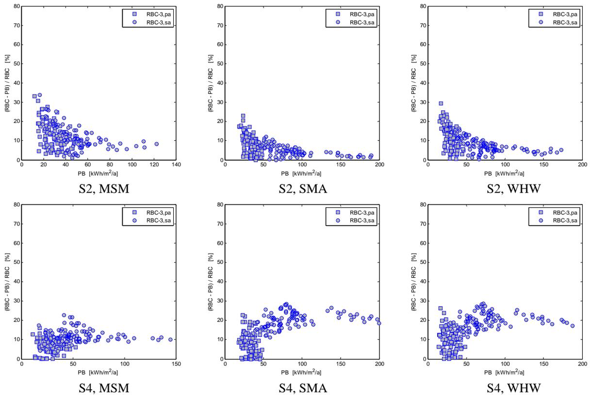
Figure 4. Relative additional annual total NRPE usage for control algorithm RBC-3 compared to the PB.
