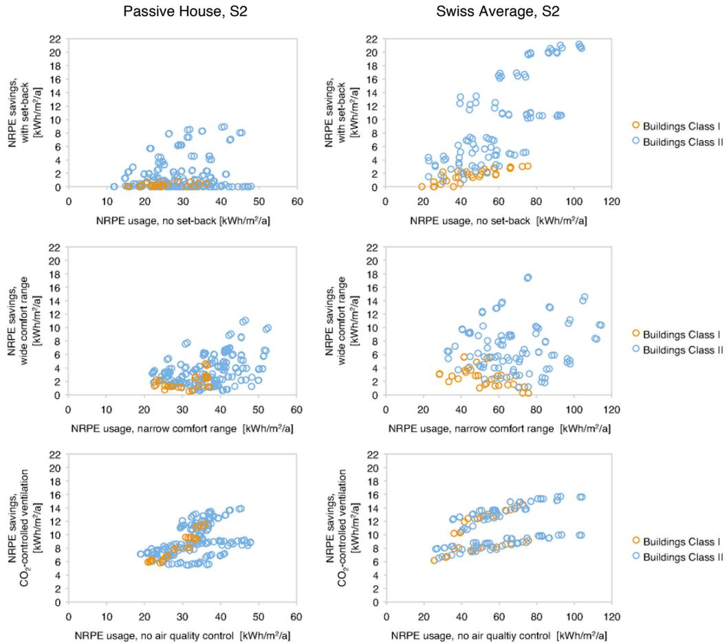
Figure 3. Absolute savings potentials for annual total Non-Renewable Primary Energy (NRPE) usage and building system variant S2 as a function of NRPE base values. Shown are savings due to *a*) allowance for night/weekend room temperature set-back (top), *b*) the widening of the thermal comfort range (middle), and *c*) the use of CO<sub>2</sub>-controlled ventilation instead of non-air quality controlled ventilation (bottom).
