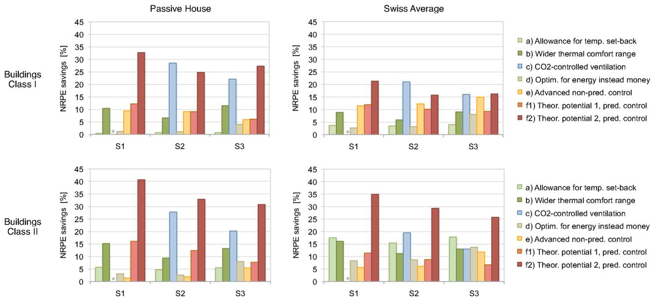
Figure 2. Comparison of average relative savings potentials for annual total Non-Renewable Primary Energy (NRPE) usage. Note, savings potentials  $a$ )– $e$ ) can be realized in practice, whereas  $f1$ ) and  $f2$ ) are theoretical values representing the maximum achievable savings given perfect predictive control. S1–S3: building system variant; \*: value not available.
