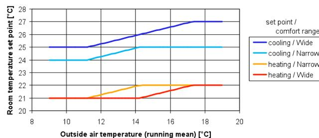
Figure 1. Room temperature set points for heating and cooling, and for the temperature comfort ranges “Narrow” and “Wide”. Reproduced from [9].
